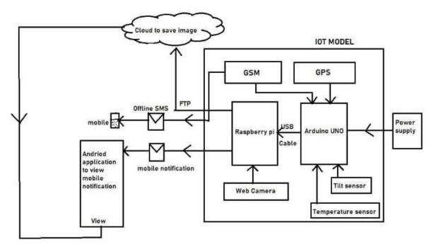
Fig 1 shows the block chart of the proposed work. The framework design contains the power supply, Arduino, temperature sensor, raspberry pi module, camera, GPS, GSM, and an emergency signal that goes about as a contribution to the gadget.
